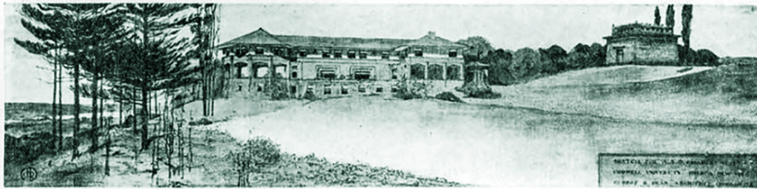
ALPHA DELTA PHI CHAPTER HOUSE AT CORNELL UNIVERSITY, ITHACA, NEW YORK. GEORGE R. DEAN, ARCHITECT, CHICAGO, IS DESIGNED TO STAND ON A POINT OF GROUND OVERLOOKING THE CITY. THE LARGE PLATE-GLASS WINDOWS IN LIVING-ROOM LOOK UP AND DOWN THE VALLEY. THE TWELVE-SIDED PORCH HAS WINDOWS THAT SLIDE UP INTO THE WALL OR MAY BE PULLED DOWN IN WINTER, INCREASING THE LIVING-ROOM SPACE. THE BUILDING WILL BE OF BRICK AND PLASTER WITH STONE BASEMENT AND TILE ROOF. THE LODGE STANDS ABOUT TWENTY FEET HIGHER ON THE GROUND THAN THE HOUSE, THE ENTRANCE BEING APPROACHED BY A FLIGHT OF STEPS
